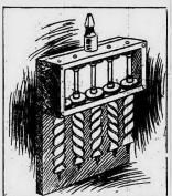
tical carpenter, aside from the fact that its cost is no more than the old ma-chine. At one side of the frame which supports the bits is a guiding plate, attached in such a manner that the turn toward or away from the bits, thus adjusting the tool for cutting the mor-tise at the proper distance from the edge of the timber, and as the bits are removable from the frame the mortise taking off one or more of the end bits.
