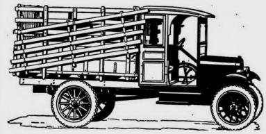
The cut shown above is a combination stock rack and stake body. Many other body types for every class of heavy hauling are made by standard body manufacturers to fit Chevrolet Utility Express Truck.
