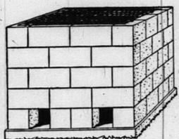
a thin layer of mortar and leaving two 8" x 8" spaces at the front to provide ample draft for complete incineration. The cover is turkey wire, 1" x 2" mesh, with welded joints so the wires won't separate due to the heat. Eye-bolts may be inserted in the joints between two of the top building blocks, if you want to hinge the mesh cover by looping down two pieces of the wire into the metal eyes.
