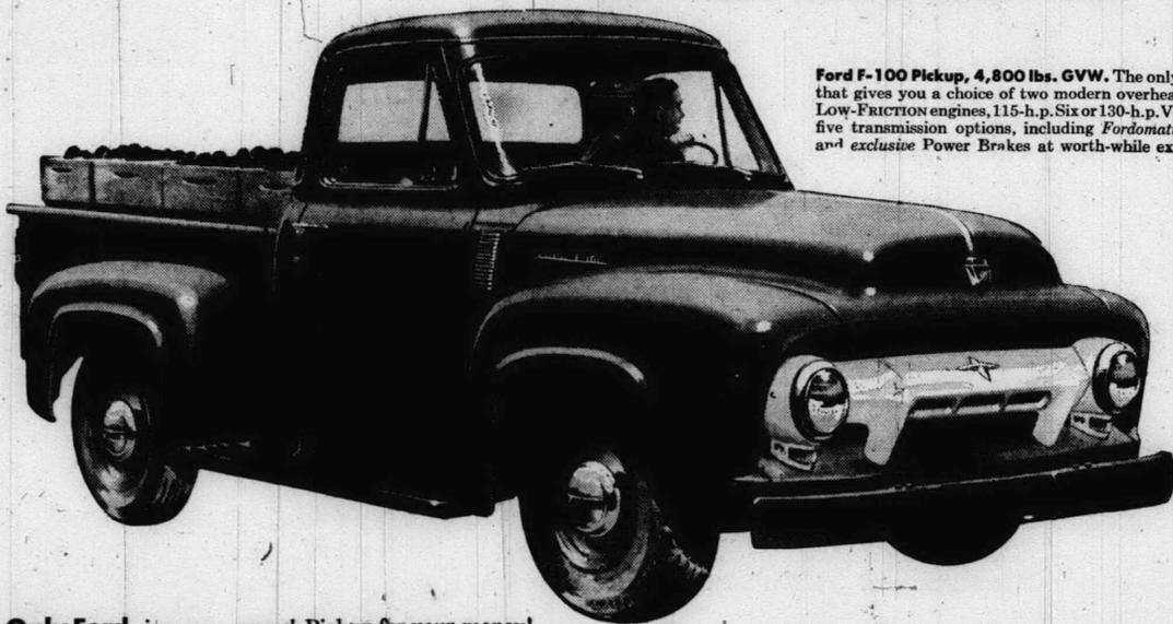
Ford F-100 Pickup, 4,800 lbs. GVW. The only Pickup that gives you a choice of two modern overhead-valve, LOW-FRICTION engines, 115-h.p. Six or 130-h.p. V-8... plus five transmission options, including Fordomatic Drive, and exclusive Power Brakes at worth-while extra cost.
