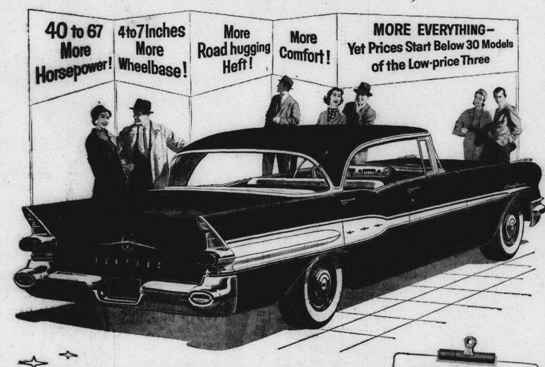
This handsome husky breaks all the rules on how a low-priced car should act! Get on the driving end and see for yourself. Feel the split-second response of its king-sized 347 cu. in., 10 to 1 compression ratio Strato-Streak V-8—the same basic power plant that shellacked 'em all in the Daytona Grand National.\* (At a little extra cost you can add
