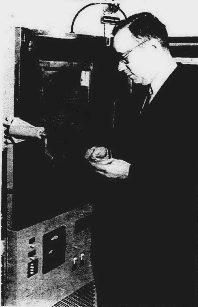
IT'S NOT FOR BAKING PIES -- This may look similar to a built-in kitchen oven, but it's actually an altitude chamber in Omni Spectra's environmental laboratory. Here, Engineer Harry Liebziet prepares to test a microwave component in the chamber to see if it will withstand altitude and humidity conditions to be experienced by an actual spacecraft.
