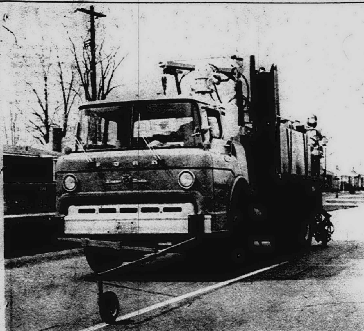
IMMEDIATE TRAFFIC — No longer will drivers on Wayne County roads have to wait several hours for the drying of the stripes of paint that mark traffic lanes. The County Road Commission has purchased a machine for nearly $31,600 that applies instantly drying paint, two lines at a time. It moves at 10 to 12 miles an hour and is followed by a supply vehicle.
