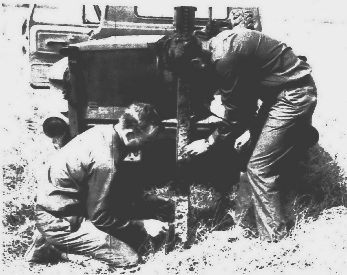
JERRY LARSON and Paul Corner examine a soil core sample taken with a hydraulic-powered soil probe in the cooperative soil survey of Wayne County. (USDA photo)
