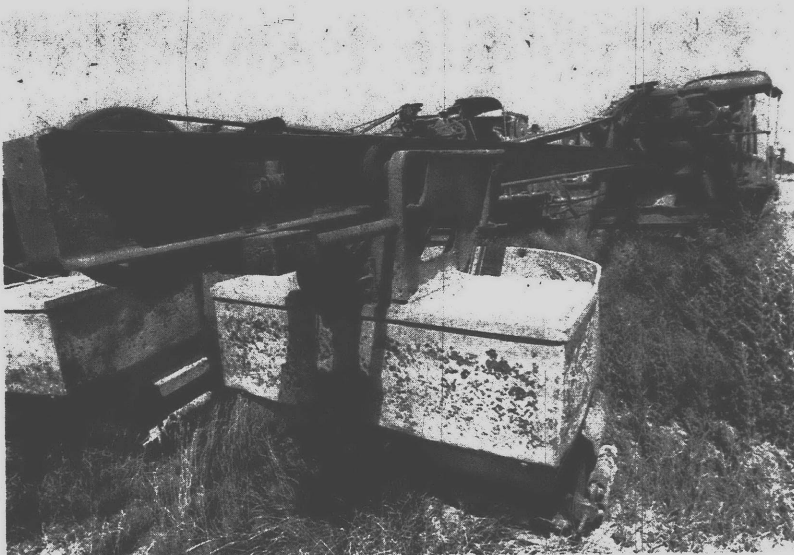
THE MACHINE with the long beam is a grade mixer and is designed to spread concrete. The dual drums mounted on the beam are operated by the cable. The machine is fed by "batch trucks" which bring dry mix to the construction site. (Observer photo by Bob Woodring)
