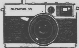
CdS meter controls electronic shutter for completely automatic exposure control. Fast 1/800 shutter and fast f/2.8 lens. Focus down to 3 feet.
