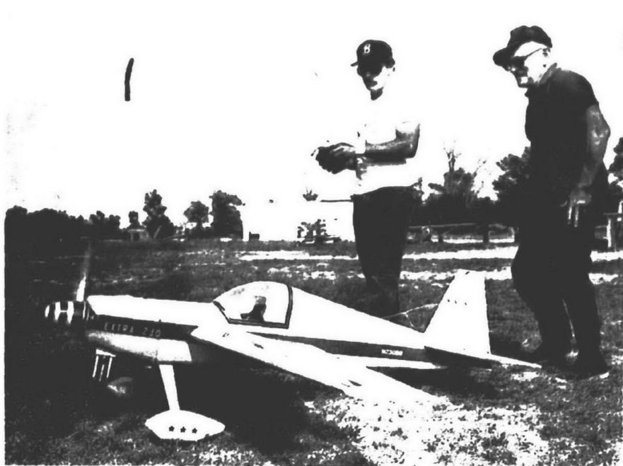
Bob Shatterow (left) taxis his Extra 230, which is powered by a modified chainsaw engine. It can fly at speeds up to 100 mph.
