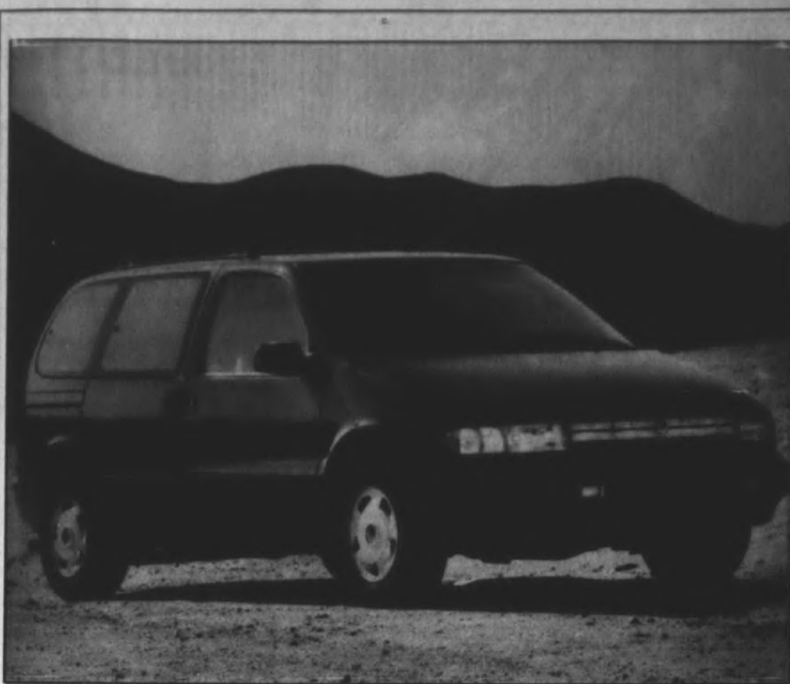
The 1993 Mercury Villager brings Ford's Lincoln-Mercury Division into the minivan market. The front-wheel drive vehicle is powered by a 3.0 liter V-6 and a four-speed automatic transmission. A flexible seating system allows 14 different seating and cargo-carrying configurations.
