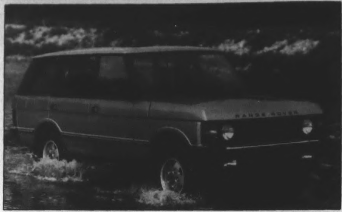
The 1993 Range Rover County LWB is the first sport utility vehicle in the world to use adjustable air suspension, which can raise the vehicle to wade through water 22 inches deep. The Rover is powered by a 4.2 liter V-8 which creates 200 horsepower. This year's Range Rover's have received more than four dozen engineering refinements.
