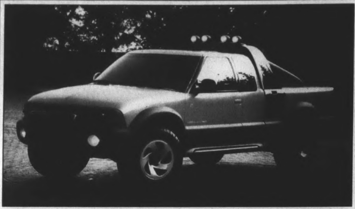
Chevrolet's Highlander "fun runner" borrows from the S-10 Extended Cab Pickup. It features a 165 hp 4.3 liter V-6, a four speed automatic transmission, a front brush bar, fog lamps, and a front and rear winch. An automatic weather "roll top," like a roll-top desk, can cover the truck bed.
