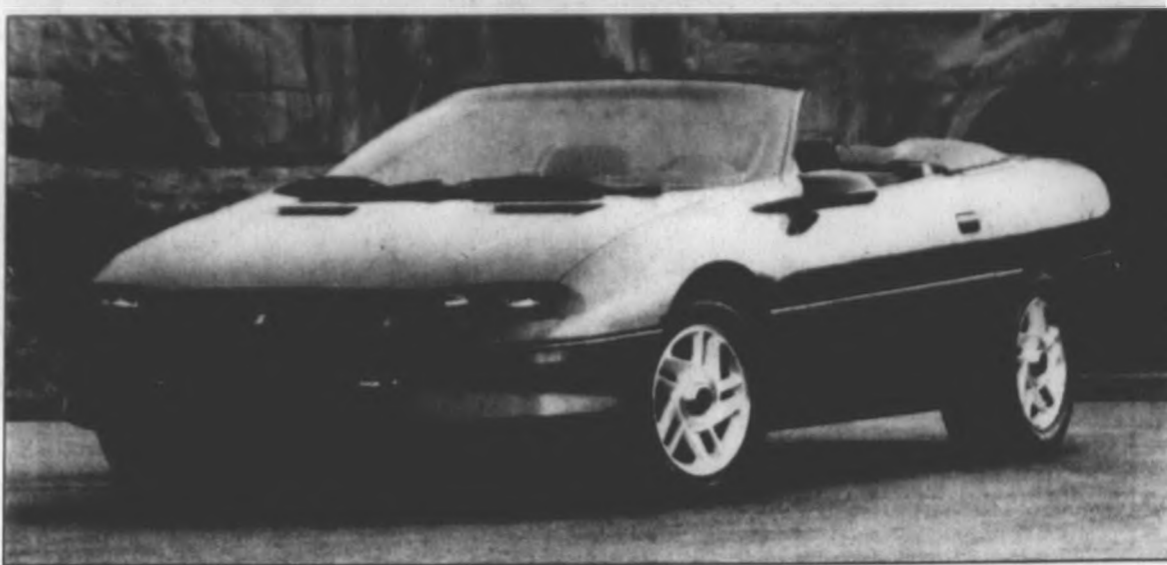
The '94 Camaro convertible power-operated top folds down flush, and a three-piece hard cover gives a finished appearance during top-down driving. It also features a full headliner and a heated glass backlight as standard equipment.
