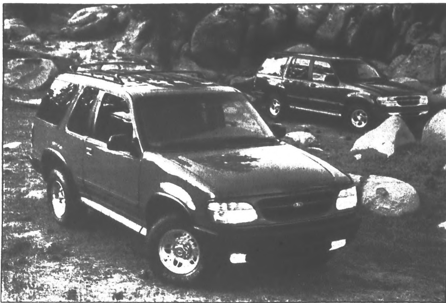
Redesigned: The Ford Explorer has been redesigned for 1995 with a sloping hood and new fenders, bumper, headlights and grille. Redesigned bodyside moldings and tail lights round out the new look. Also new is a choice of 15-inch cast aluminum or 16-inch chrome steel wheels.
