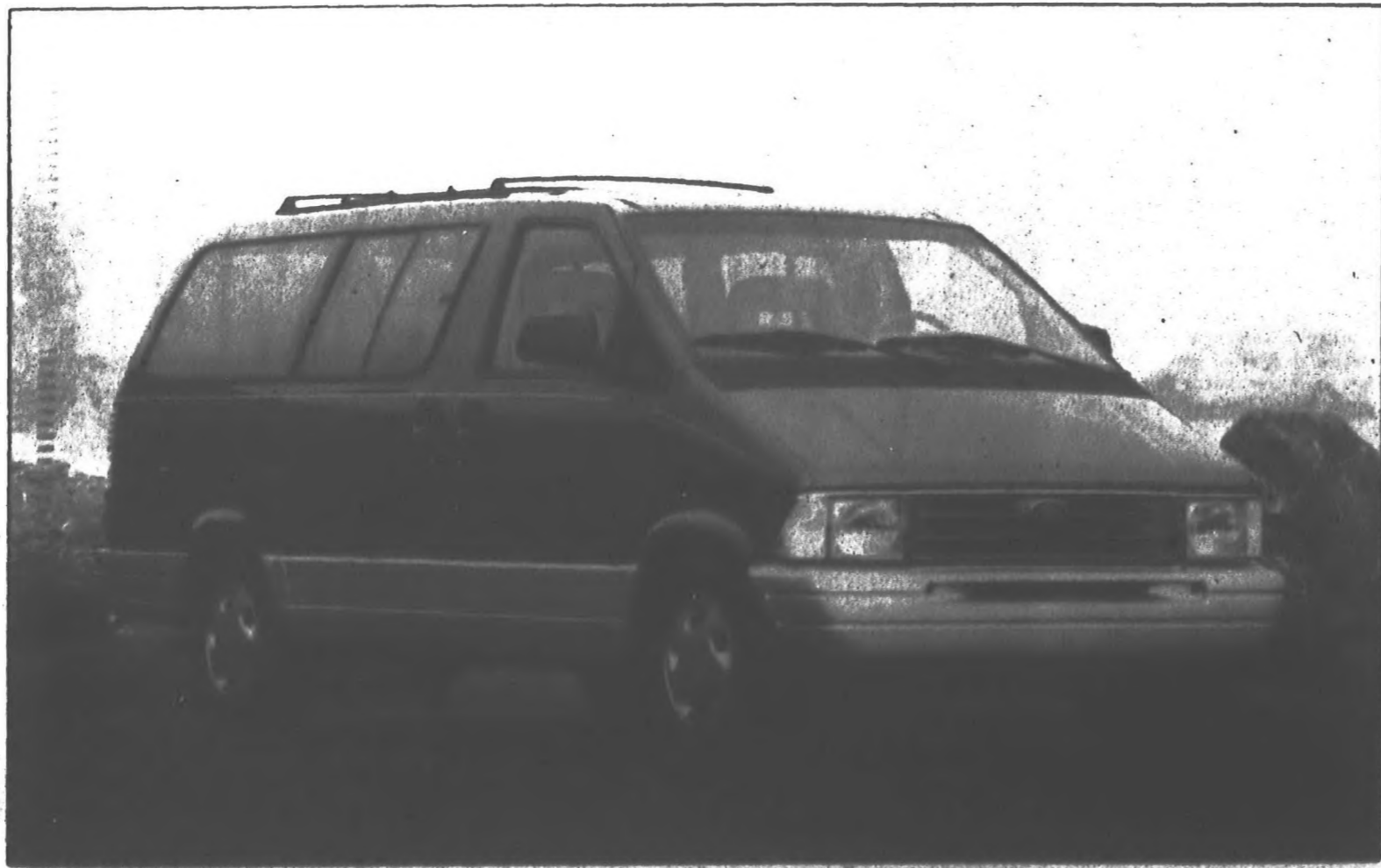
Aerostar: The Aerostar minivan offers a seven-passenger wagon and cargo van with a new occupant protection feature. Side-door guard beams joining the driver's side airbag and rear anti-lock brakes as standard equipment. There are two power plants: 4.0-liter and 3.0-liter V-6s.
