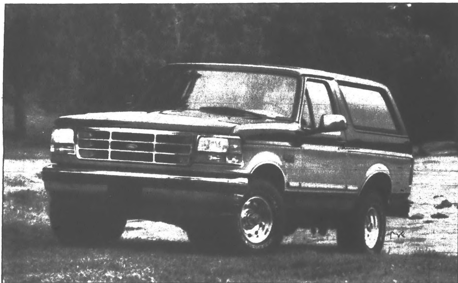
Bronco choices: Bronco models are powered by either of two electronically fuel-injected V-8 powerplants. The 5.0-liter motor can be teamed with either a five-speed manual transmission or a four-speed automatic. The 5.8-liter V-8 is paired exclusively with the automatic.
