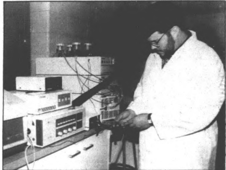
At work: Phillip Beauchamp, a Plymouth resident, (below) is evaluating the molecular weight distribution of a polymer using gel permeation chromatography. Brandy Alderson, (above) a Westland resident, prepares a solvent sample for odor evaluation.
