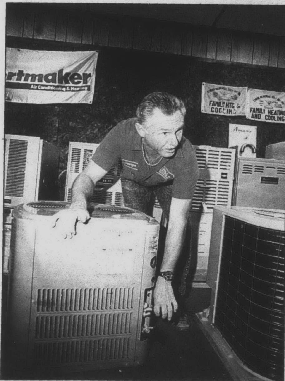
Leak potential: George Klempert, owner of Family Mechanical, Heating, Cooling & Electrical in Garden City and Madison Heights, points out where freon gas is most likely to leak, over time, at the compressor connection.
