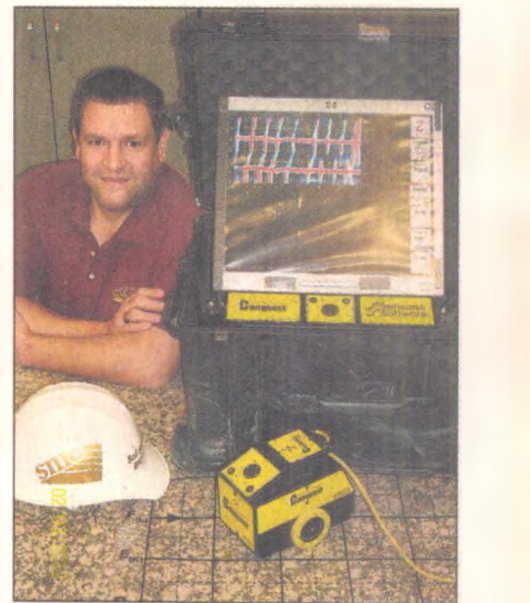
Civil engineer Keith Toro of Canton Township with the impulse radar unit that helped him "see" beneath the sidewalks on Georgia Street in downtown Indianapolis. Toro works for Soils and Materials Engineers Inc. in Plymouth Township.
