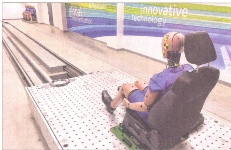
It's a short but real fast ride for the test dummies in the new Johnson Controls sled-test lab. This new sled can deliver about 700,000 pounds of force. BILL BRESLER | STAFF PHOTOGRAPHER
