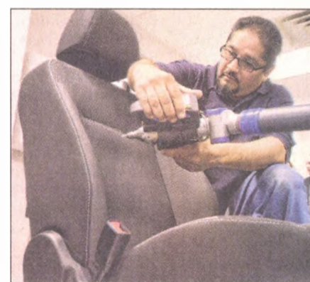
Jaime Yanez of Taylor uses a laser scanning device to create a virtual copy of a car seat in a JCI laboratory. Dan McCosh (right) is an automotive industry journalist.
