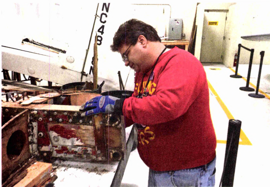
Chris Curran of Allen Park scrapes paint metal parts on the wing where it attaches to the fuselage. SUE MASON
